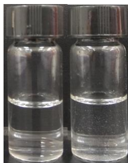
Figure 3. The images of OSA with: pH > 10 (on the left) and pH < 4 (on the right)
