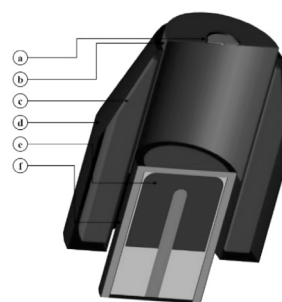
Fig. 3 The MCNP model of the CSS in 3D construction. (a) radioactive source, (b) sample mount, (c) annular BGO crystal, (d) aluminum cover of BGO detector, (e) germanium crystal, (f) aluminum cover of HPGe detector.
