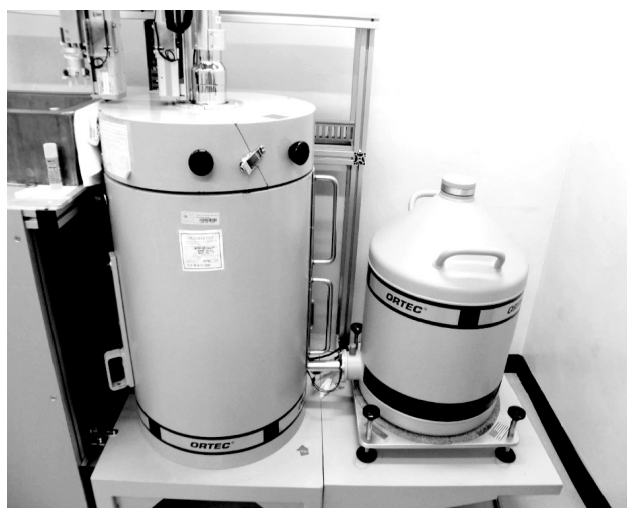
Figure 1. (top) the schematic diagram of Compton suppression system. (bottom) the photograph of the CSS at NAA's lab.
