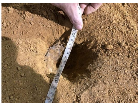
Fig. 7. Measurement of explosion chamber parameters.
