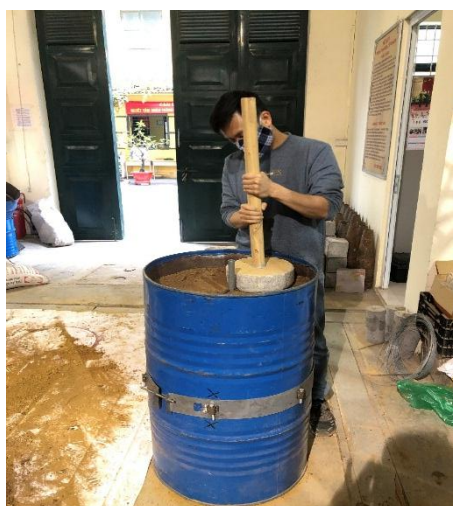
Fig. 3. Compact the soil.
