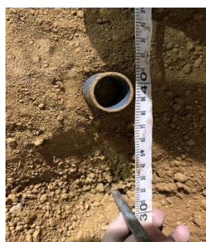
Fig. 8. Sampling to determine post-explosion tightness.
